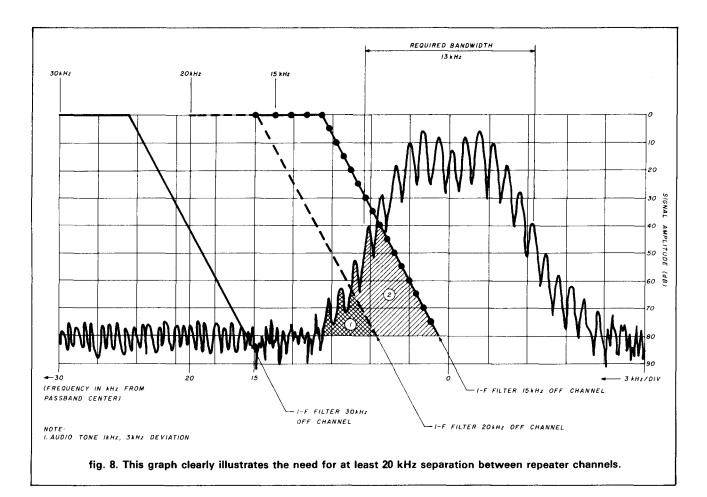
Finally, when these results are compared with the EIA specification for minimum acceptable adjacent channel rejection, we see that all the receivers failed the test at 15 kHz spacing, and all but the handheld unit passed the test at 20 kHz spacing (see appendix).
